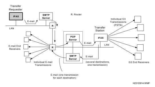
The requesting terminal dials the Transfer Station, and requests it to transfer the message to end receivers stored as quick dials, speed dials, and group dials in the Transfer Station.
