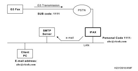
When a G3 fax message is received with a SUB code (max. 20 digits), the machine compares this SUB code with the Personal Box SUB codes stored in the machine with e-mail addresses. If there is a match, the machine routes the message to that e-mail address by e-mail.
